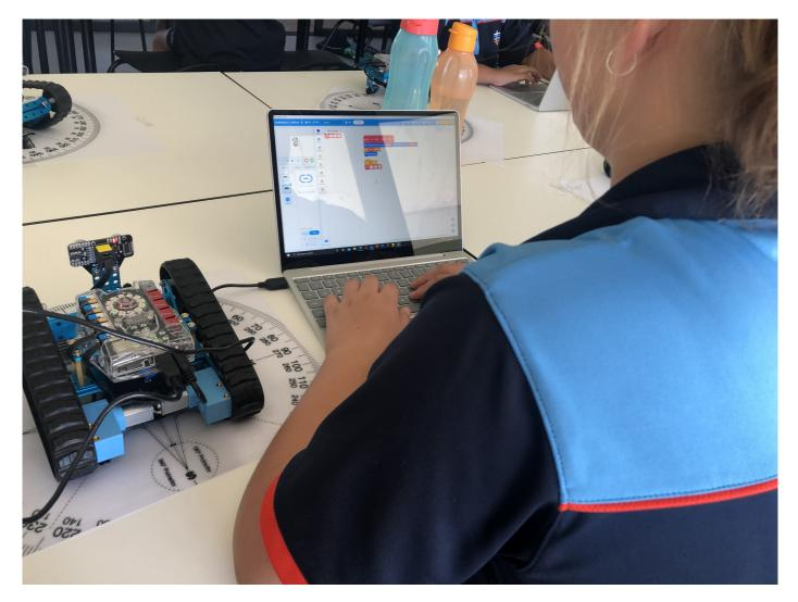
In the Coding and Robotics elective the Year 8 students have been investigating how to code an mBot Ranger to perform basic movements. Using block code, students have successfully driven their robots forward and made them turn. One of the challenges that students faced was making the robot turn a fixed number of degrees. Using the gyroscope was proving difficult, and the software does not have a command to perform a 90° turn.
